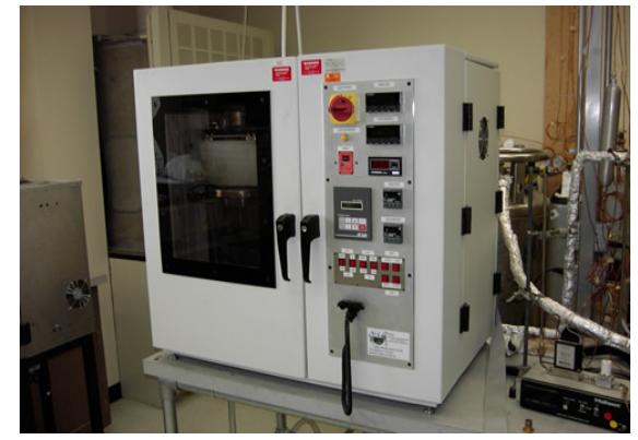
CREC Riser Simulator allows for the development of new catalysts for the cracking and reforming of diverse hydrocarbon feed stocks which is a major breakthrough for the manufacture of clean fuels. Professor Hugo De Lasa heads the CREC research and consulting laboratory that develops new reactor technologies in close collaboration with the industrial sector. Ten CREC Riser Simulators are used across the world today.
