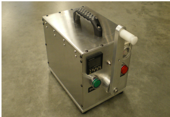
Dip Apparatus was designed for the department of dentistry. The dip apparatus sweeps from one side to the other dipping it's sample in various environments for repetitive heat cycle testing. With variable cycle and dwell times, this unit was designed to run forever. We ran 50,000 cycles here in our shop before delivery.
